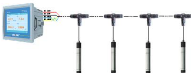
Diagram 7.5 Field data bus serial application
