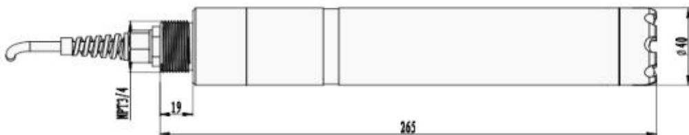
Diagram 6.1 Physical size drawing (Unit: mm)
