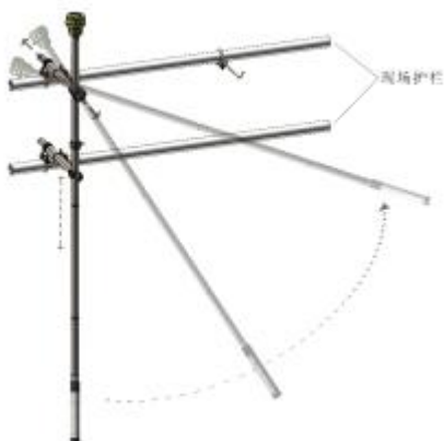
Diagram 7.1 Environmental protection bracket installation
